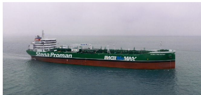
Fig. 5. Stena Pro Patria, a dual-fuel methanol vessel owned by Proman and Stena Bulk 40
